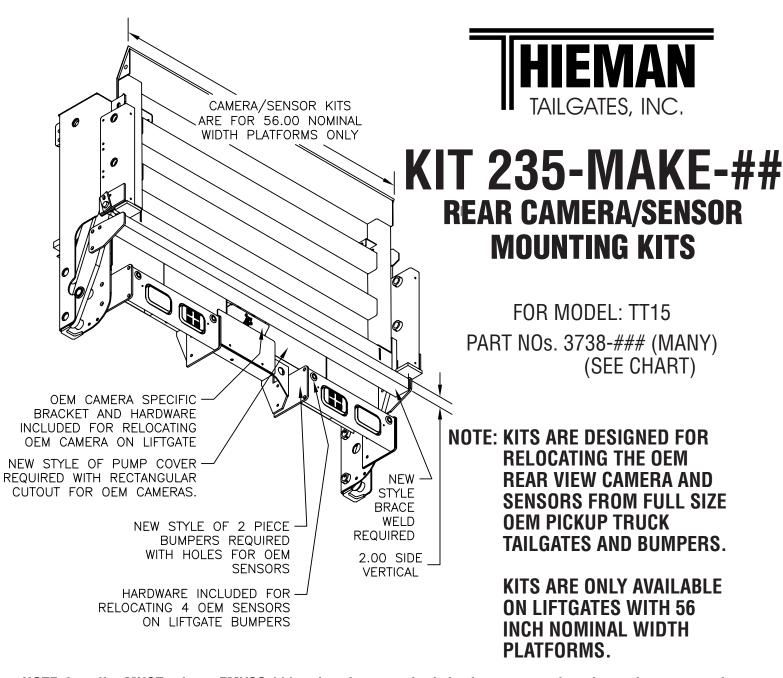
NOTE: Installer MUST refer to FMVSS 111 and perform required checks to ensure the relocated camera conforms. WARNING: Relocated OEM camera will have a different point of view, which will affect screen guidelines. Relocated sensors may perform differently in the relocated positions. Make sure to check surroundings and mirrors prior to reversing vehicle.
